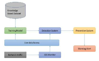
Figure 1: IDS Working on IoT.
